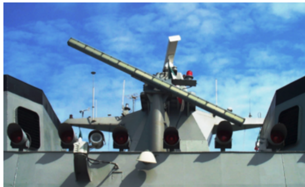
Figure 4.2: Gyro-stabilized reference bar used for approach and landing.
